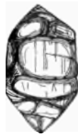
FIG. 69.—Magnified section of an olivine crystal; the light portions represent the undecomposed mineral, the shaded parts show the conversion of the olivine into serpentine.
